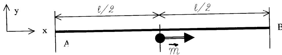
$$\begin{aligned}\vec{m} &= m\hat{x} \\ \vec{m}_A &= \vec{m}_B = -m/2\hat{x}\end{aligned}$$
