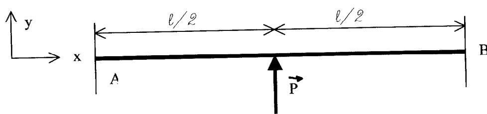
$$\begin{aligned}\vec{P} &= P\hat{y}: \\ \vec{RA} &= \vec{RB} = -P/2\hat{y} \\ \vec{m}_B &= -\vec{m}_A = P\cdot\ell/8\hat{z}\end{aligned}$$
