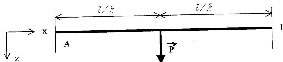
$$\begin{aligned}\vec{P} &= P\hat{z}: \\ \vec{RA} &= \vec{RB} = -P/2\hat{z} \\ \vec{m}_B &= -\vec{m}_A = -P\cdot\ell/8\hat{y}\end{aligned}$$
